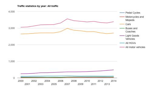
As both sets of figures and graphs show, traffic in and out of Callander has maintained a similar level between 2000 and 2014 apart from 2007/2008 which saw a steep increase, particularly on the A81 between A873 and A84. This increase has, however, once again levelled off, and has actually decreased slightly.
