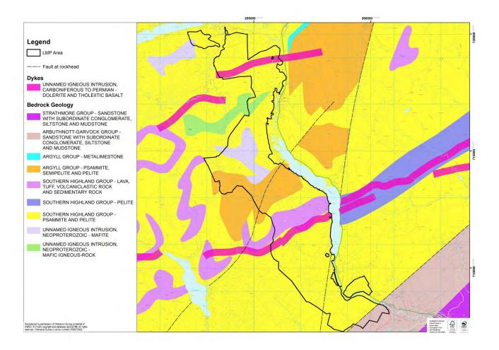
The underlying geology follows the grain of the Highland fault to the south, with a more complex geology over the northern part of the LMP area.
